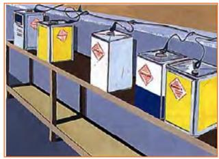
Fig.3.1.15: Earthed containers to store flammable solvents
